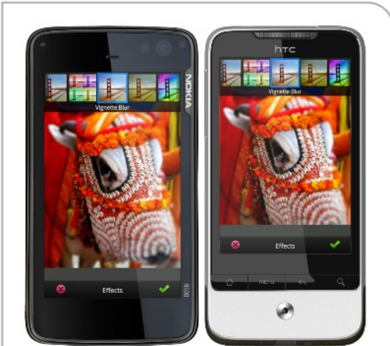
Figure 2 : Alien Dalvik running Android Photoshop on Nokia N900 vs native application on HTC legend
